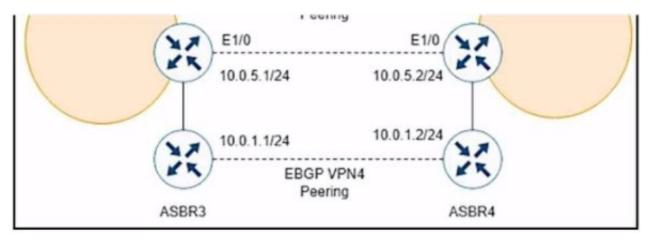
While troubleshooting, a network engineer discovers that the backup path fails between ASBR3 and ASBR4 for traffic between BGP AS6000 and BGP AS6500 when the connection between ASBR1 and ASBR2 goes down. The following configurations were performed on ASBR1:
